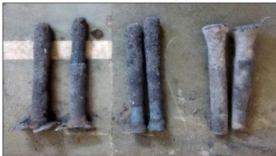
Fig. 10: As – cast specimen (from left) in green sand mold, dry sand mold and CO<sup>2</sup> mold
