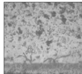
Fig. 14: Microstructure of CO<sup>2</sup> sand mould
