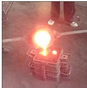
Fig. 4: Pouring of molten metal
