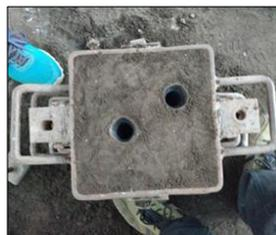
Fig. 7: Dry sand mould
