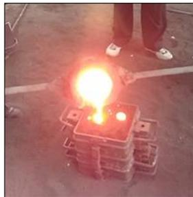
Fig. 4: Pouring of molten metal
