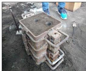
Fig. 6: Green sand mould
