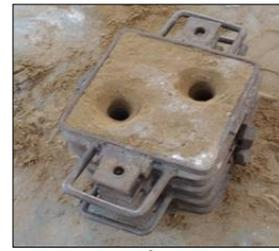
Fig. 8: CO<sup>2</sup> sand mould
