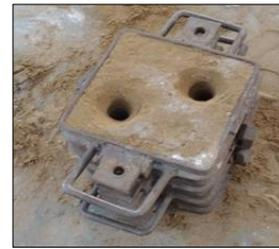
Fig. 8: CO<sup>2</sup> sand mould
