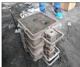
Fig. 6: Green sand mould
