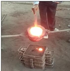
Fig. 3: Fe-Si alloy addition
