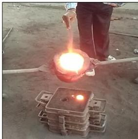
Fig. 3: Fe-Si alloy addition
