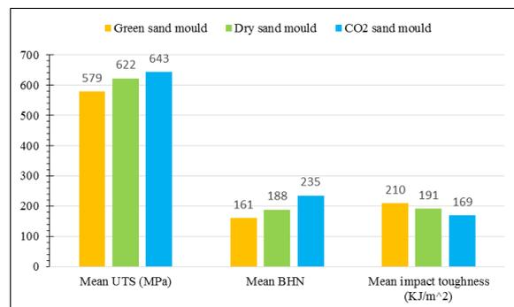
Fig. 15: Comparison among the different sand moulds
