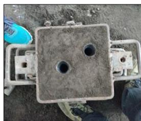
Fig. 7: Dry sand mould
